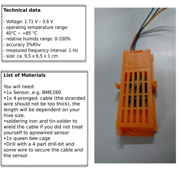
The BME280 does not only measure the relative air humidity. It can also measure temperate and air pressure. The BME280 is controlled over the 12C Bus or SPI.
